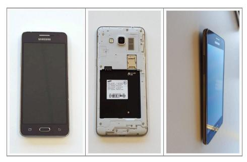
**Grade D**: Devices will contain some degree of liquid damage. Devices will power on, but may have cracked screens or housing, gaps between housing, LCD damage. Devices may have issues with charging/battery life. Suitable for component harvesting.
