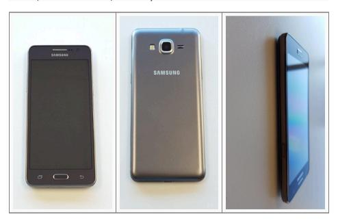
**Grade C**: Functional unit. Will have at least one of the following conditions: cracked screen or housing, liquid damage, gaps between housing, gouges, LCD damage, customization, bad audio codec. The unit's originally installed software may have been rooted. Phones may have issues with charging / battery life.
